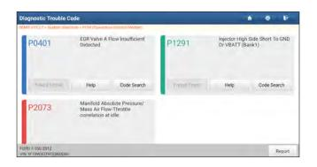
Warning: Retrieving and using DTCs for troubleshooting vehicle operation is only one part of an overall diagnostic strategy. Never replace a part based only on the DTC definition. Each DTC has a set of testing procedures, instructions and flow charts that must be followed to confirm the location of the problem. This information can be found in the vehicle's service manual.
