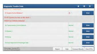
The tested system with fault code appears in red and the system with OK displays in green (normally).
