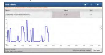
• Min/Max: Tap to define the maximum/minimum value. Once the value goes beyond the specified value, the system will alarm.
